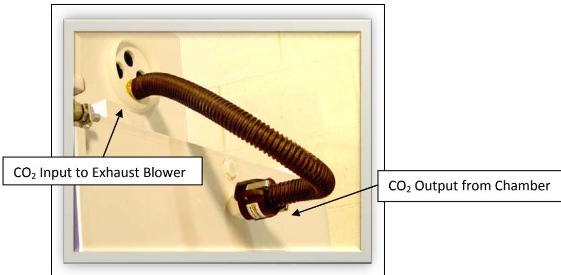
5) Attach the 1" intake hose from the blower to the "CO<sub>2</sub> Out" on the right side of top chamber. The clamp connector fastens by pulling the two clamps away from chamber.
