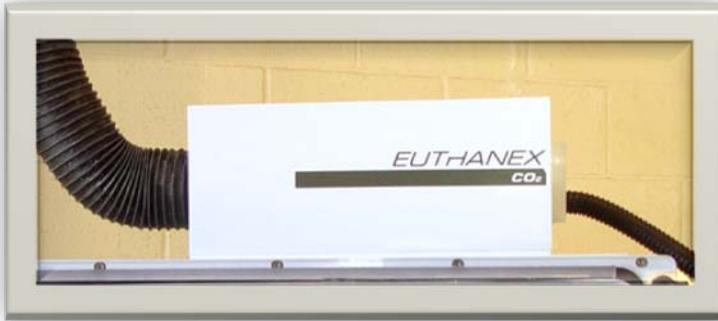
4) Rest the exhaust blower on top of the chamber. The large 4" exhaust hose must be on left and the 1" intake hose on the right.
