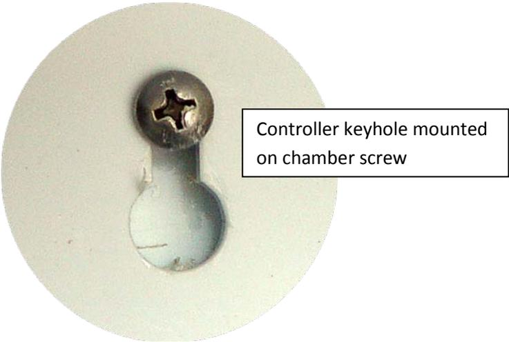
Align the keyholes with the four screws on the left side of the chamber. Push in and slide down to secure. The screws may be tightened for permanent mounting.
