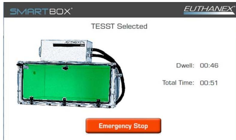
The red emergency “STOP” button may be pressed at any time to stop the euthanasia cycle. A password may be required to engage the stop (admin setting). Gas will immediately stop flowing and the unit will purge.
